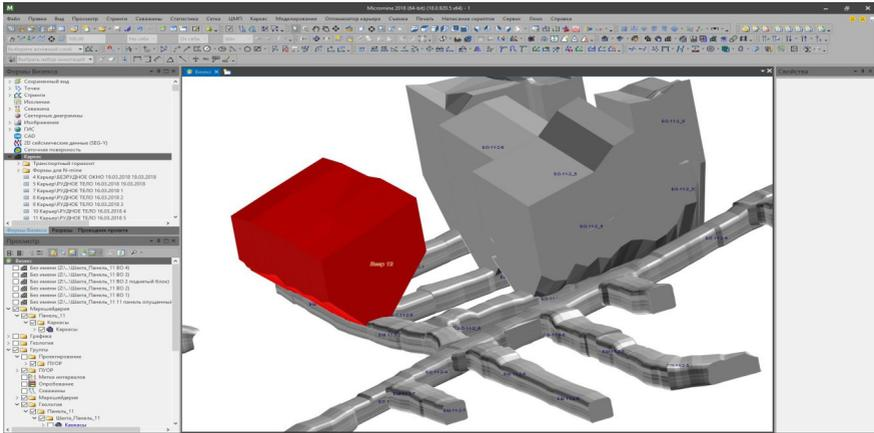
**Fig. 3.** General view of the frame model for mining the ore deposit of poor copper - nickel ores in the Micromine software window
